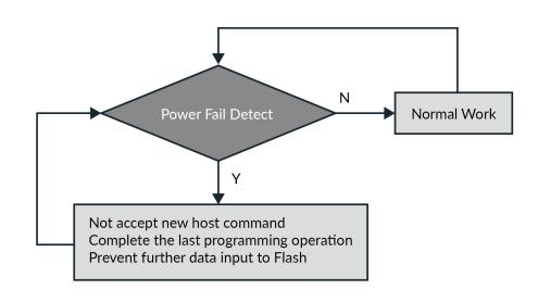
Figure 1: Power Failure Data Protection Block Diagram of Innodisk SSDs
